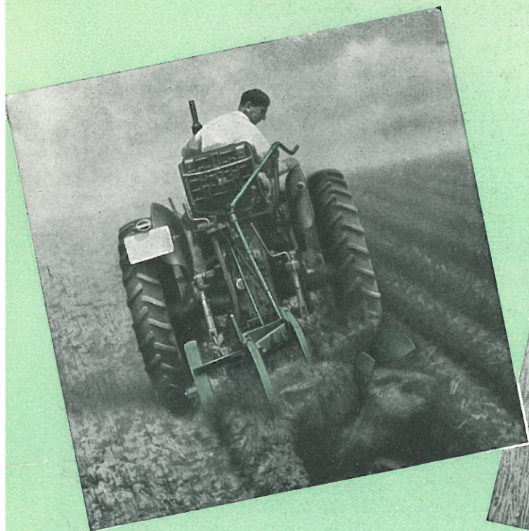
THE PN 252 TWO-BOTTOM MOUNTED PLOUGH is a sturdy type designed for deep ploughing up to 11 in. Its cutting width is 23\frac{3}{4} in. The depth is controlled from the driver's seat. It is equipped with 2 skim coulters and a disc coulters. The bottoms are of general purpose type.
